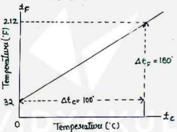
If  $t_c$  and  $t_f$  are temperature values of a body on Celsius temperature scale and Fahrenheit temperature scale respectively, then the relationship between Fahrenheit and Celsius temperature is given by
