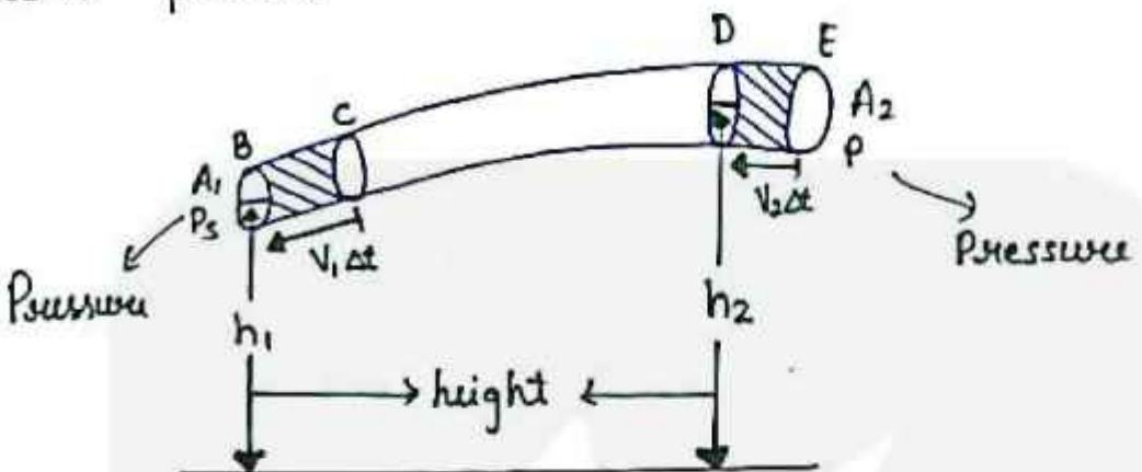
Movement of fluid from V<sub>1</sub>,Δt to V<sub>2</sub>,Δt in Δt time interval.
